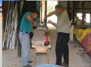
While Truman and Gene prepared the rail by drilling the ends to accept the rail joiners . . .
